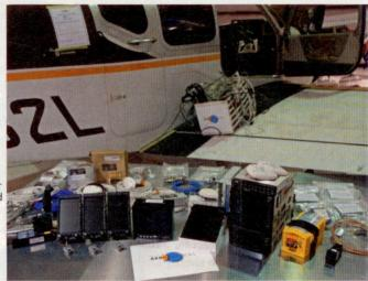
Now for some interesting new twists. Alpha Systems has provided the airplane with its angle-of-attack (AOA) indicator. The indicator's fast-slow indicator will be mounted right on the glareshield—right in the pilot's field of view, and mounted just like the AOAs you see in military airplanes or business jets. Fly an approach with the AOA's target "doughnut" lit up, and you'll be on speed for every landing. It's a feature that any pilot will greatly appreciate.
